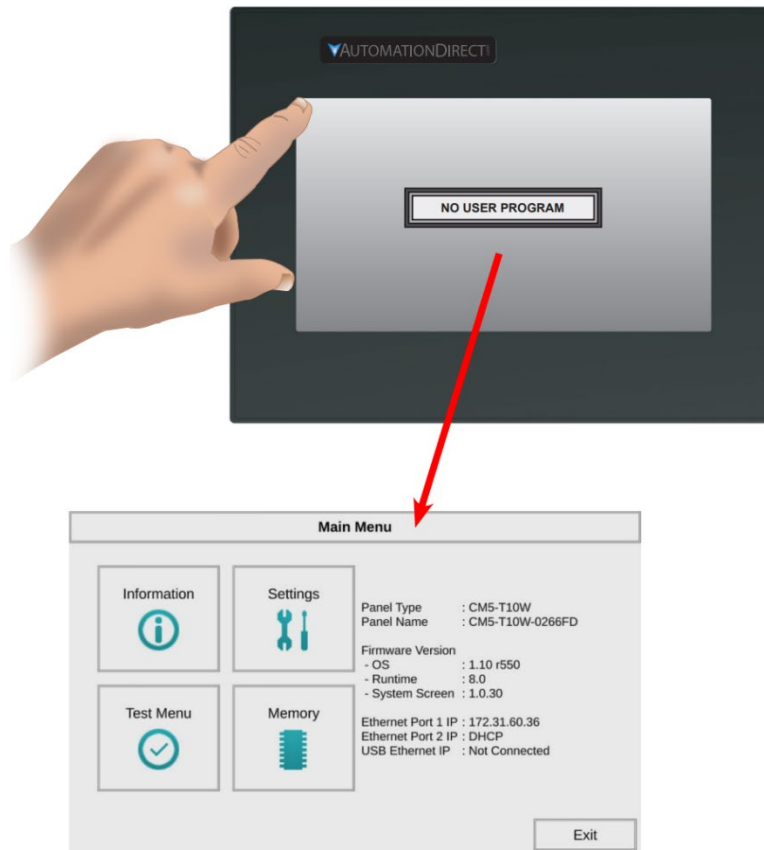
Figure 14 – Accessing the System Setup Screen
